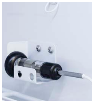
Temperature sensor in glycol bottle
